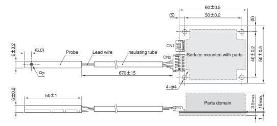
CN1 S4B-PH-KLC-H(LF)(SN) JST Connector (I/O pins) 1: GND(Vcc)
