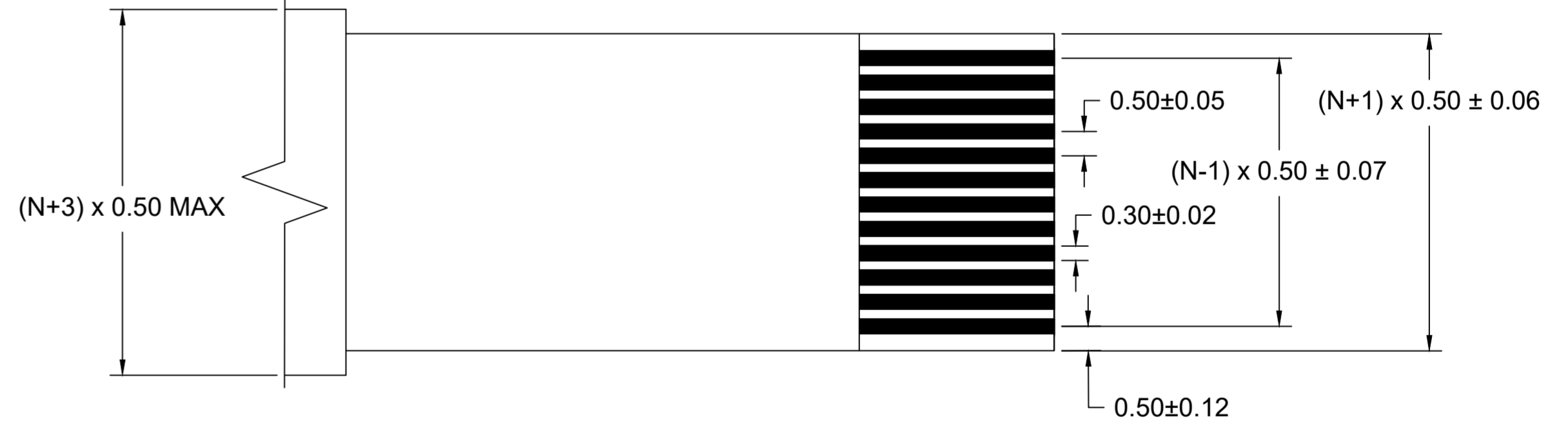
END-TAIL DIMENSIONS SCALE 10:1
