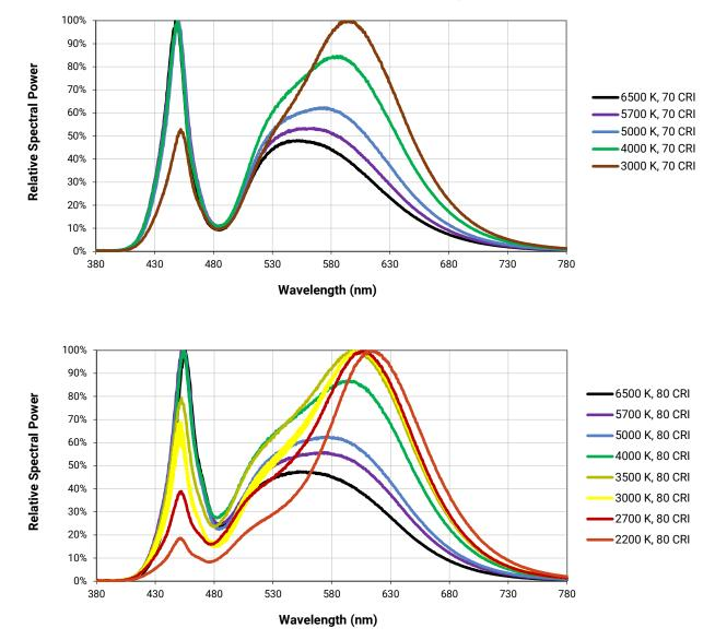
The following graphs are the result of a series of pulsed measurements at 1620 mA and  $T_{J}$  = 85 °C.
