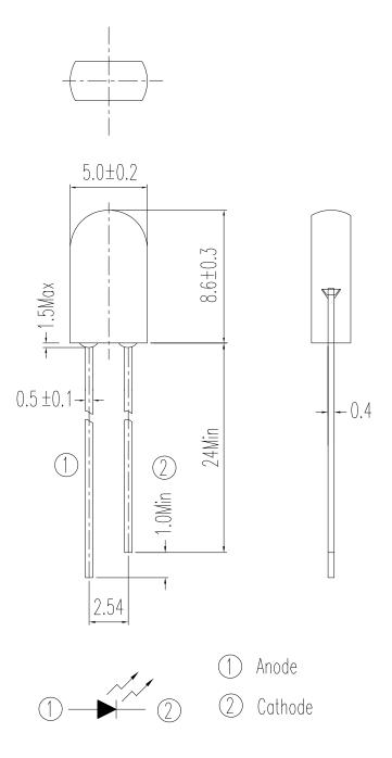
Note: Tolerances unless dimensions ±0.25mm
