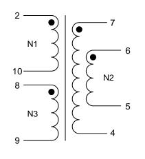
N2 dentotes two windings connected in parallel. Terminals  $4\!+\!5$  and  $6\!+\!7$  must be tied as solder bridging is allowed.
