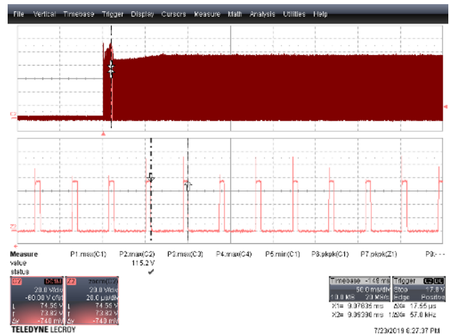
Figure 44 – Drain Voltage and Current Waveforms. V_{IN} = 400 \text{ VDC} , I_{OUT} = 2.5 \text{ A} . V_{FWD(MAX)} = 115.2 \text{ V} Upper: V_{FWD} , 20 V, 50 ms / div. Bottom Half: Zoom @ 20 \mu\text{s} / div.
