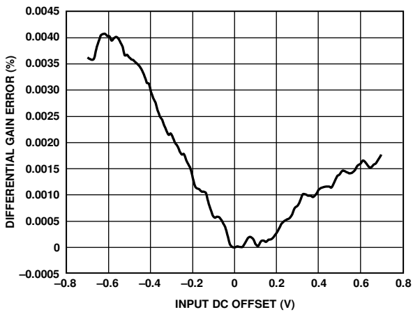
Figure 45. ADV3228 Differential Gain Error
