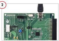
Ensure that shunt is placed between 5 V and VCC of jumper J1. Plug in the USB cable to the CY3280-20x66 Universal CapSense Controller Board.
