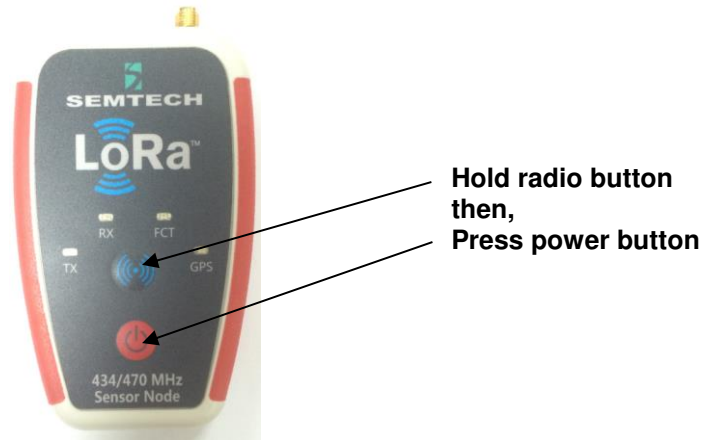
Figure 9: How to enter bootloader mode with LoRa Sensor Node
