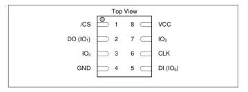
Connect the clip to the flash, oriented with the red cable on pin 1. For example this is the clip connected to the flash on a ESP8266 board:
