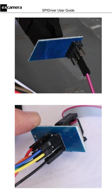
and connect the clip cable pins to the SPIDriver like this:
