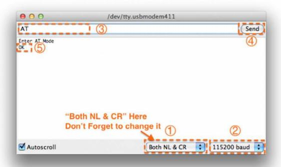
Fig1: enter the AT command, remember selectting the Both NL & CR
