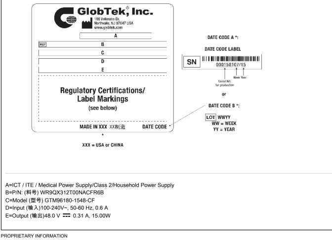
PROPRIETARY OF GLOBTEK, INC. ANY REPRODUCTION, DISCLOSURE OR USE OF THIS DRAWING, IN WHOLE OR IN PART, IS HEREBY PROHIBITED EXCEPT AS SPECIFIED IN WRITING BY GLOBTEK, INC. © GlobTek, Inc. 2019 - 2023 guest / 08/03/2023 2:35:41 AM GMT CLONED FROM WR9QI625T00NACFR6B
