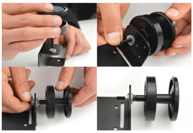
Step 3: Insert the motor into the bracket and tighten it with 3 M3\*6 flat head screws.
