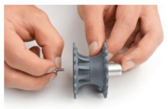
Step 5:Install the drive wheel on the motor and tighten with black screw; please note: the hole on the coupling must be aligned with the flat end of the motor shaft.
