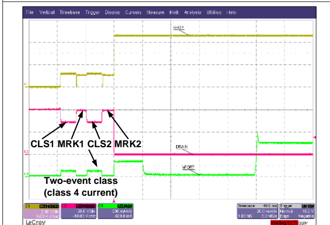
Figure 55. Two-event Classification (Class 4) and Power On
