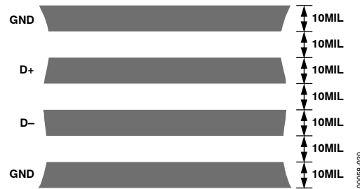
Figure 20. Arrangement of Signal Tracks
