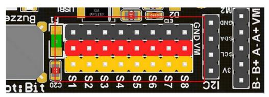
Robotbit extension has also built-in blocks for DC motors and steppers. With onboard cell you may drive 4x TT motors or 2x 28BYJ steppers, or a mixture of theese. Keep in mind that VM may out 2A to motors and servos. If you use external source please keep the input around 5V or less, a high voltage external input may damage the 5V boost circuit.
