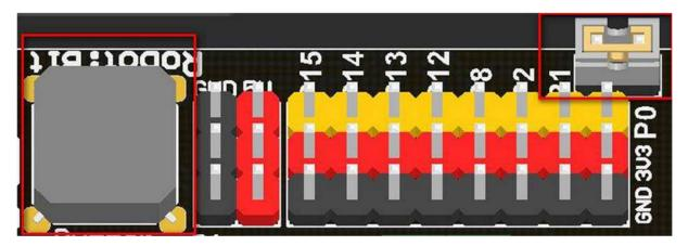
The buzzer jumper cap is plugged in by default, and the corresponding buzzer is connected to the Micro:bit P0 port. If you need P0 for other purposes please unplug the jumper. The buzzer associate to music blocks in makecode.
