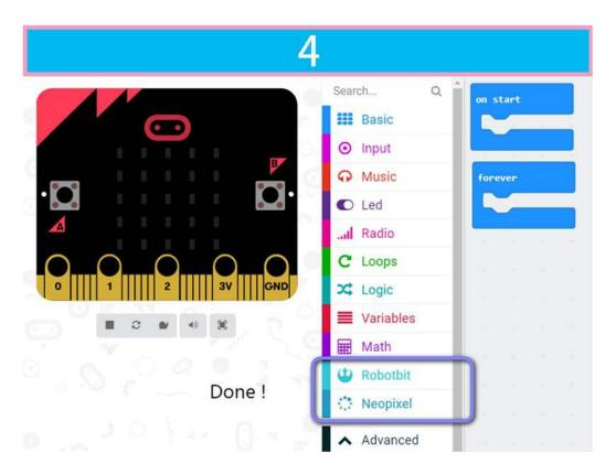
Drag some of the robotbit blocks out to workspace, remember to connect the corresponding motor servos, etc.
