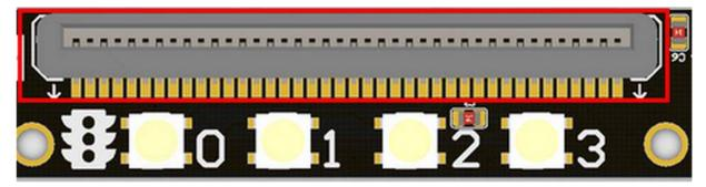
For installing Microbit mainboard. Please install Microbit with led matrix and RGB led in the same direction.
