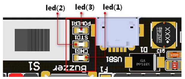
Led(3) is the power indicator, will be always on after switch is turned on. Led(1) is charging indicator, will be on while charing and Led(2) be on once fully charged.
