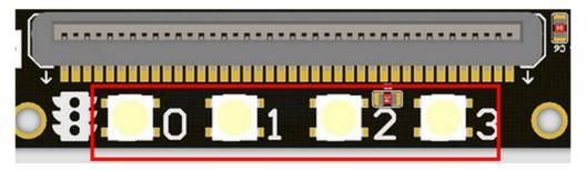
The robotbit extension for makecode has integrated neopixel support. Neopixel array connect to P16 of microbit.
