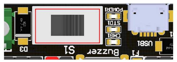
Turn on the switch (in the direction of green terminal input), will provide onboard 3.3V 5V and VM(motors and servos directly driver by battery cell)
