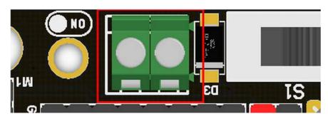
Although there is anti-reverse protection, but still pay attention while wiring. The positive and negative silkink of this interface is on the back of Robotbit. You can only input 5V or less into this port. If you have a higher voltage source you may need a LDO or DC-DC module to buck the voltage down.
