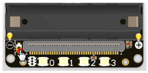
Once you got your RobotBit extension board please first install a 18650 battery, pay attention to the positive and negative pole (even we have anti-reverse protection). You have to activate the power management system by pressing the Battery Act push button. Each time you switch a battery cell or let the power management go into protection mode (over current or over discharge), you have to redo this step.
