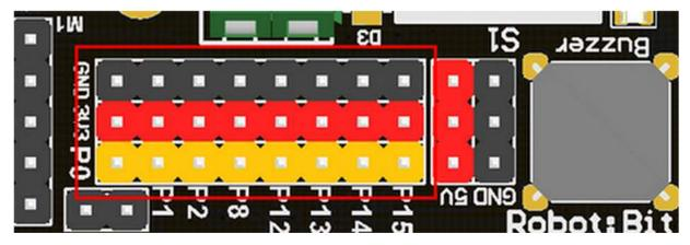
We have released P0-P2 \ P8 \ P12-P15 from Microbit to Robotbit for common IO usage. P0~P2 has analog read/write support, others may act as digital IOs. You may connect commonly modules for Arduino to Robotbit, there is also 5V output in case your module only support 5V power input. Please note that Microbit IO signal level is 3.3V.
