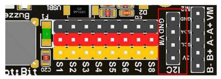
Expandable I2C module, can only be used to plug in I2C module.
