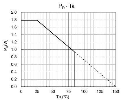
When mounted on the board (JEDEC 4 layers)
