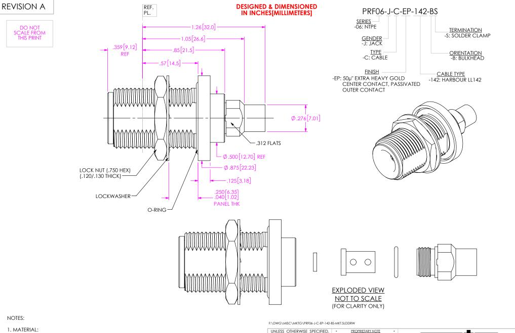
BODY, BUSHING, CLAMP NUT, LOCK WASHER, JAM NUT: STAINLESS STEEL CONTACT: BERYLLIUM COPPER SOLDER FERRULE: BRASS ALLOY BEADS: PEI O-RINGS: SILICONE RUBBER
