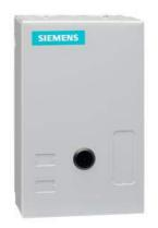
Non-reversing NEMA contactor, Size 0, Three phase full voltage, Contactor amp rating 18A, 3 wire (NO aux included), 240V 50Hz / 277V 60Hz coil, Non-combination type, Enclosure NEMA type 1, Indoor general purpose use, Standard width enclosure
