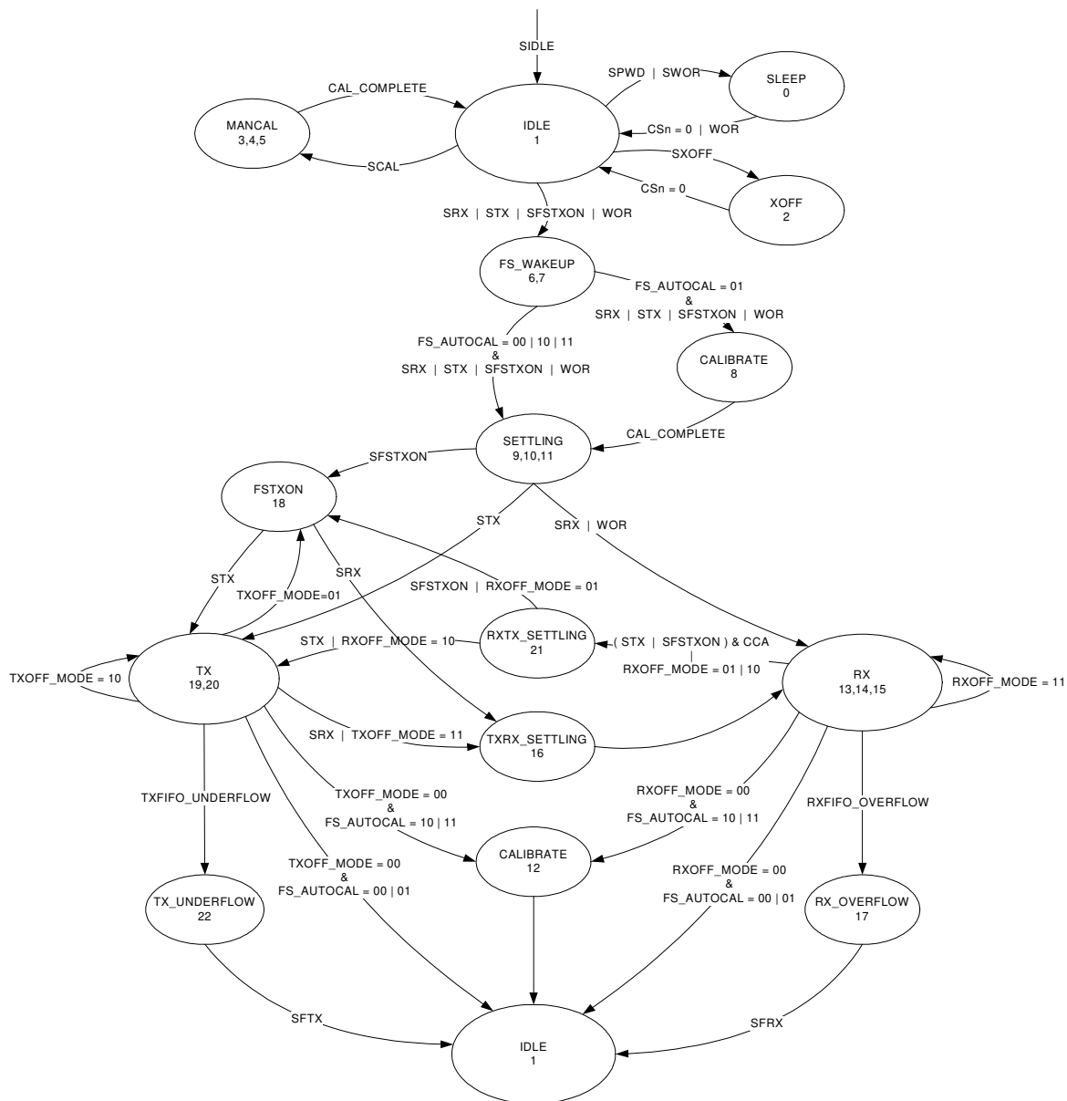
Figure 20: Complete Radio Control State Diagram
