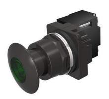
30mm BlackMax, Epoxy Coated Corrosion Resistant Complete Metal Unit Illuminated Push-Pull Operator Transformer type, 240V AC Incandescent Lamp Mushroom Head Cap Small 1 3/4" (44.5 mm) Metal, Black with Green Lens 3 Position Pull-Momentary/Push-Maintained UL Listed, CSA Certified NEMA 1,3,3R,4,4X,12,13 & Automotive Standards
