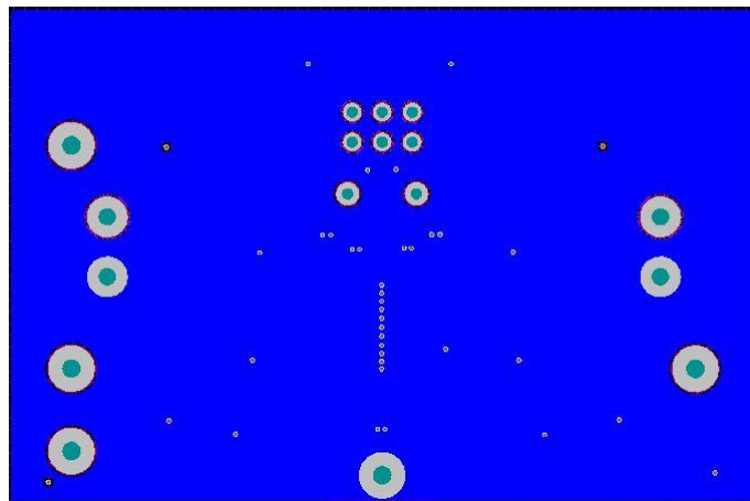
Figure 2. PCB Copper Layout & Silk Screen – Bottom
