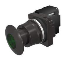
30mm BlackMax, Epoxy Coated Corrosion Resistant Complete Metal Unit Illuminated Push-Pull Operator Transformer type, 480V AC Incandescent Lamp Mushroom Head Cap Small 1 3/4" (44.5 mm) Metal, Black with Green Lens 3 Position Momentary UL Listed, CSA Certified NEMA 1,3,3R,4,4X,12,13 & Automotive Standards
