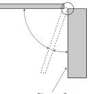
Diagram B The damper torque becomes larger, preventing the lid from closing completely
