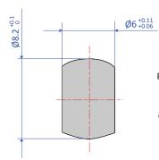
Recommended dimensions for mounting a rotating shaft
