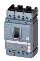
circuit breaker 3VA5 UL frame 250 breaking capacity class H 65kA @ 480 V 3-pole, line protection TM230, FTAM, In=150A overload protection Ir=150A fixed short-circuit protection Ii=5...10 x In UL489 SB (naval), 50 deg. cel. cable connection on both sides
