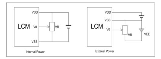
VDD-V0: LCD Driving Voltage VR: 10k-20k
