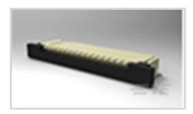
Connector System: Flex-to-Board Number of Positions: 27 Centerline (Pitch): 1 mm [.039 in ] Insertion Force Type: Zero Insertion Force (ZIF) PCB Mount Orientation: Right Angle
