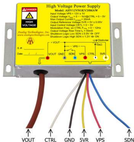
Figure 2. The Connecting Lead Wires of AHV12VN1KV20MAW
