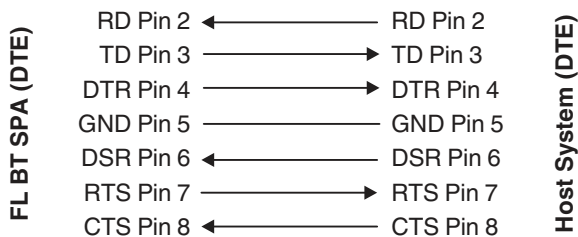
Figure 8 Assignment of 1:1 cables
