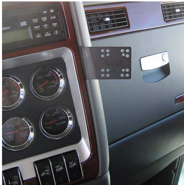
InDash installed showing location
