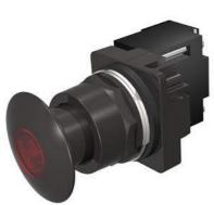
30mm BlackMax, Epoxy Coated Corrosion Resistant Complete Metal Unit Illuminated Push-Pull Operator Full Voltage, 6V AC LED Lamp Mushroom Head Cap Small 1 3/4" (44.5 mm) Metal, Black with Red Lens 3 Position Pull-Momentary/Push-Maintained UL Listed, CSA Certified NEMA 1,3,3R,4,4X,12,13 & Automotive Standards
