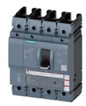
circuit breaker 3VA5 UL frame 250 breaking capacity class H 65kA @ 480V 4-pole, line protection TM230, FTAM, In=90A overload protection Ir=90A fixed short-circuit protection Ii=5...10 x In N conductor unprotected without connection
