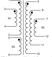
N1, N2 denotes two and three windings connected in parallel. Terminals 1+2, 3+4, 7+8+9 and 10+11+12 must be tied as solder bridging is allowed.
