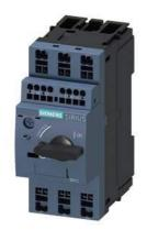
Circuit breaker size S00 for motor protection, CLASS 10 A-release 0.9...1.25 A N-release 16 A Spring-type terminal Standard switching capacity with transverse auxiliary switches 1 NO+1 NC
