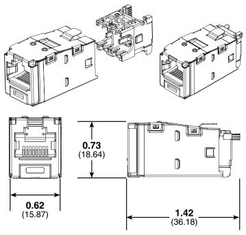
Dimensions are in inches (Dimensions in parenthesis are metric)
