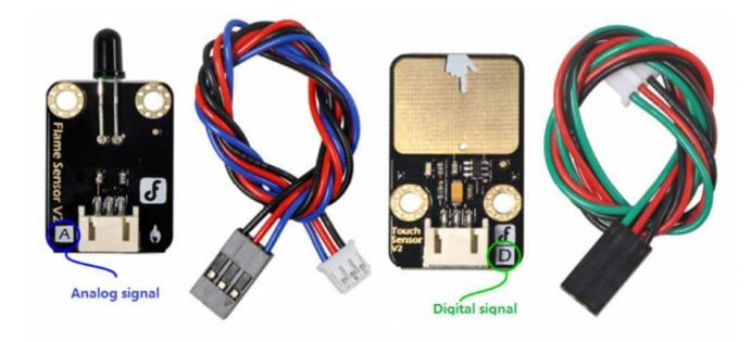
• This is DFRobot's **Gravity Interface**. Digital and analog connections are easy to recognize and support most of DFRobot's I/O expansion shields and modules. Search "**Gravity**" in the DFRobot store to find compatible modules.
