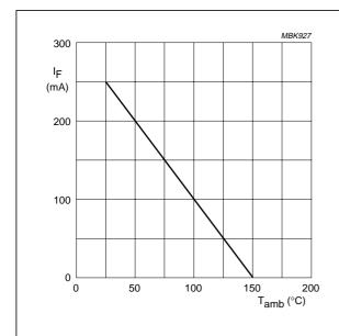
Device mounted on an FR4 printed-circuit board.
