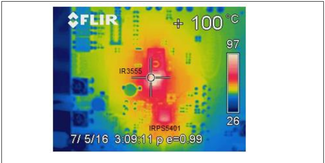
Figure 71 IR3555 thermal image
