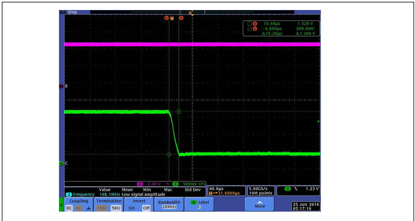
Figure 23 PINK=SM_ALERT#, GREEN=VOUT, After Enable is de-asserted, VOUT drops from 1.5 V to 0.27 V in 15 µs TOFF_FALL is 1 ms, Fixed_OVP_Thresh=1.35 V, VOUT=1.5 V
