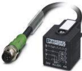
Sensor/Actuator cable, 3-position, PUR halogen-free, Black-gray RAL 7021, Plug straight M12, A-coded, on A valve plug, with 1 LED, connected with Z diode, Cable length: 1 m
