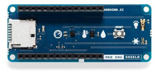
To help you build projects and store the data collected locally, this shield has a slot for a microSD card (not provided).
