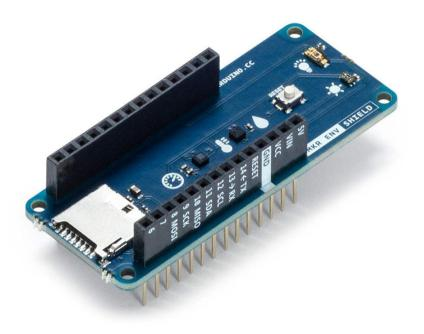
The MKR ENV Shield allows a MKR board to acquire environmental data collected by an array of sensors.
