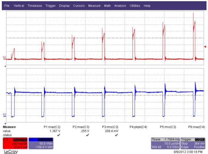
Figure 51 – 132 VAC, 60 Hz Start-up. Upper: I_{DRAIN} , 200 mA / div. Lower: V_{DRAIN} , 50 V, 10 μs / div.
