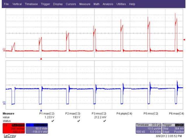
Figure 49 – 90 VAC, 60 Hz Start-up. Upper: I_{DRAIN} , 200 mA / div. Lower: V_{DRAIN} , 50 V, 10 μs / div.
