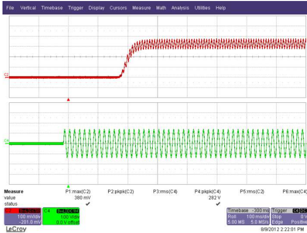
Figure 40 – 90 VAC, 60 Hz. Upper: I_{OUT} , 100 mA / div. Lower: V_{IN} , 100 V, 100 ms / div.
