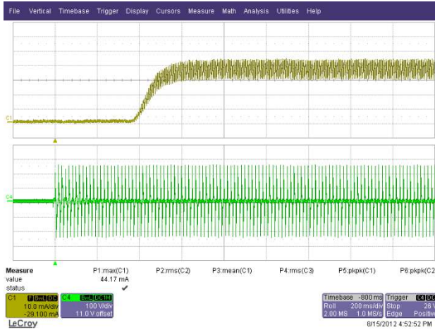
Figure 70 – 120 VAC, 60 Hz. Upper: I_{OUT} , 10 mA / div. Lower: V_{IN} , 100 V, 200 ms / div.
