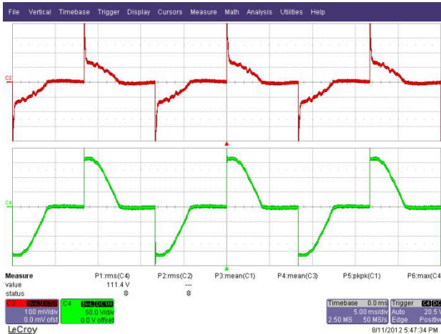
Figure 64 – 90° Conduction Angle. Upper: I_{IN} , 100 mA / div. Lower: V_{IN} , 50 V, 5 ms / div.
