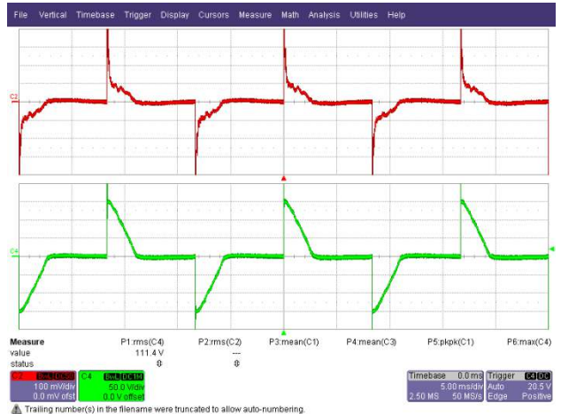
Figure 65 – 54° Conduction Angle. Upper: I_{IN} , 100 mA / div. Lower: V_{IN} , 50 V, 5 ms / div.
