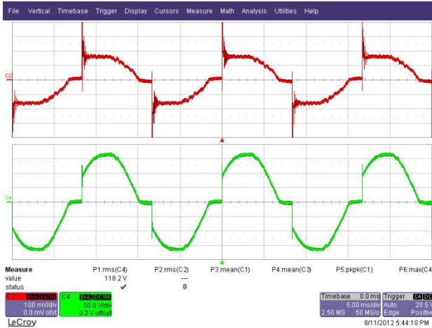
Figure 62 – 147° Conduction Angle. Upper: I_{IN} , 100 mA / div. Lower: V_{IN} , 50 V, 5 ms / div.
