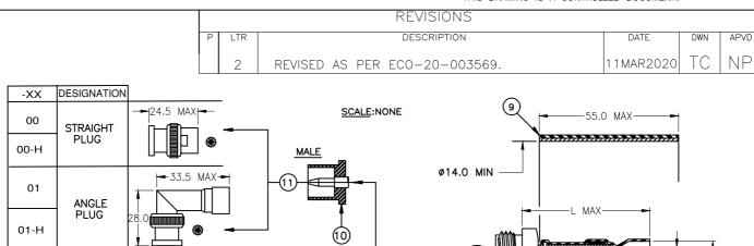
BULKHEAD JACK **FEMALE** (5)25.4 MAX† **STRAIGHT JACK** FOR EXAMPLE: RTD-50-P-00 PRODUCT DIMENSIONS CABLE DIMENSIONS 25.4 MAX + ØF MAX øΕ øG ØA MIN ØB MIN ØD MAX **STRAIGHT** L MAX PANEL 7.2 2.1/5.0 3.5/7.0 31.0 5.1 1.25 3.7 **JACK** ∠4 x M25 x 0.45
