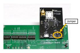
Insert a CC2538-CC2592EM board into the SmartRF06EB as shown above.
