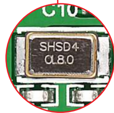
Figure 6-1: 8MHz crystal oscillator module (X1)
