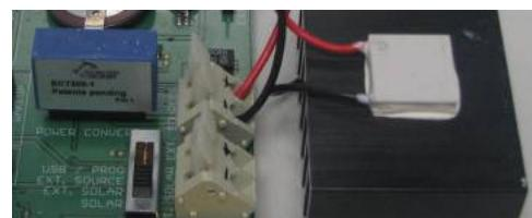
If heat sink has room temperature (e.g. 20°C) and you press one finger on the Peltier element above, the element will generate a few mV. ECT 300 will transform this to higher voltage and load short term capacitor on EVA 320. STM 300 will be powered by this energy and send telegrams.
