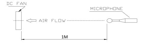
NOISE IS MEASURED AT RATED VOLTAGE IN FREE AIR IN ANECHOIC CHAMBER WITH B & K SOUND LEVEL METER WITH MICROPHONE AT A DISTANCE OF A METER FROM THE FAN INTAKE.
