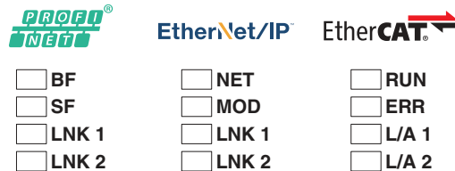
Figure 30 LED status indicators for PROFINET, EtherNet/IP™, EtherCAT®
