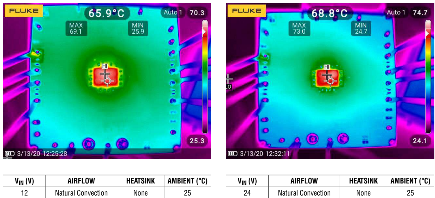
Figure 5. 12V IN and 24V IN Measured Thermal Captures with 3A Load on Each Output
