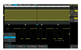
The SDS2000X-E can search events specified by the user in a frame. It can also navigate by time (delay position) and historical frames.
