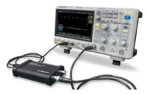
The optional 25 MHz function/arbitrary waveform generator is operated from the USB host connection. Functions include Sine, Square, Ramp, Pulse, Noise, DC and 45 additional built-in waveforms. The arbitrary waveforms can be accessed and edited by the SIGLENT EasyWave PC software.
