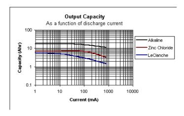
The efficiency of a carbon zinc or alkaline battery improves as the current drain decreases as seen in the above graph. As a result, an important application guide-line should be considered: "For increased efficiency, use as large a battery as possible, consistent with the physical limitations of the device." This has the same effect as lowering the current. As an example, doubling the size of a carbon zinc battery will more than double the service life at a given drain.
